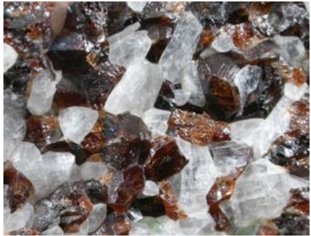
Wollastonite (white) and grandite garnet (brown) from Lewis Mine in Willsboro, NY
