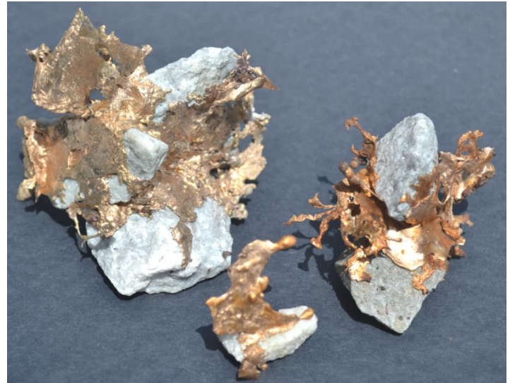
Copper fulgurites from satellite tower off of Rose Road. Largest specimen is 3: high.
