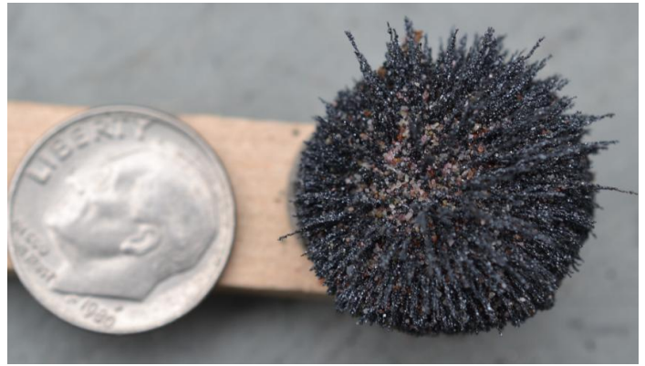
Magnetite garnet sand from Area 5 of Hamlin Beach resting on a round magnet
